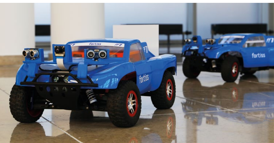
Figure 31. Fortissimo rover hardware platform – model vehicle equipped with 3D-printed components, raspberry pi controllers and sensor technology.
