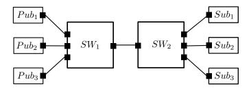
Fig. 1. Network topology with Publishers (Pub) and Subscribers (Sub) connected via a single link  $(SW_1 \ {\rm to} \ SW_2)$
